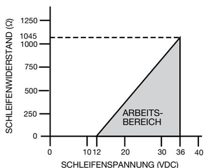
$$V_{\min} = 12 \text{ V} + [0,022 \text{ A}^{(1)} * R_L]$$
